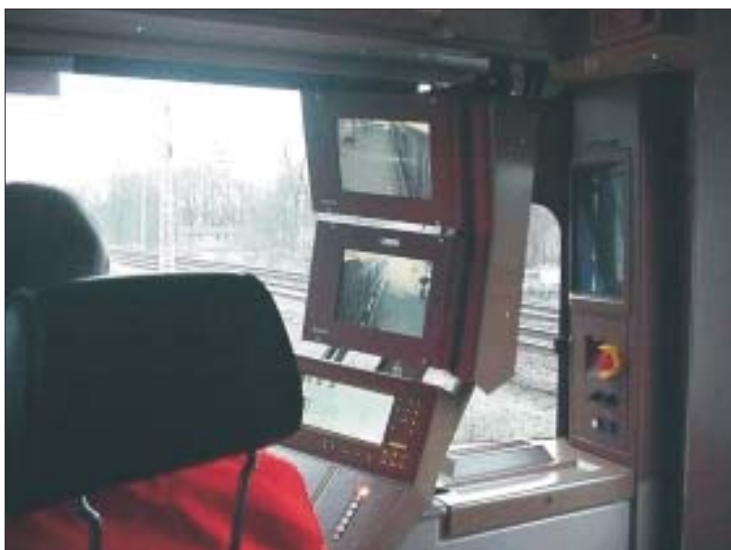
Fig. 2 • S-Bahn Berlin GmbH line S1 driver's cab with IR receiver and two TFT monitors (receiver upside the driver)
