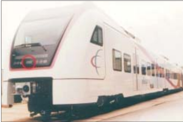
Fig. 5 • Express Rail Link KLIA in Kuala Lumpur IR receiver between the headlights
