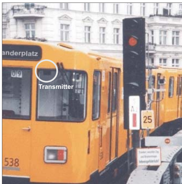
Fig. 1 • Driver's cab with IR transmitter
