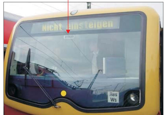
Very small Optical Receiver behind the windshield
