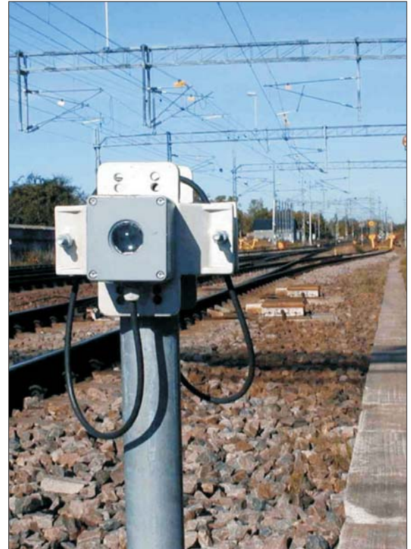
LB 200 - one way light barrier in case IP 65
