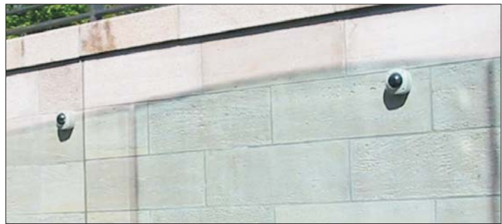
Receiver 30° in dom-camera-housing
